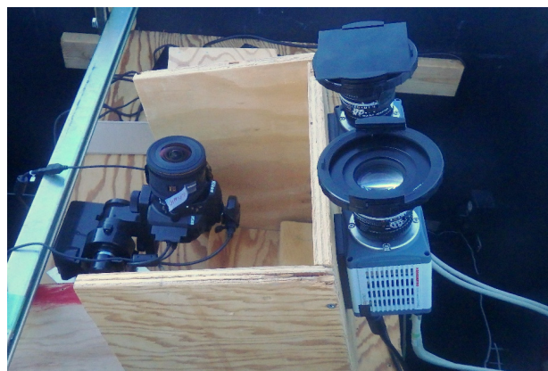
Figure 2: Automatic of burst-mode aurora imaging system assisted by all-sky DSLR camera.
