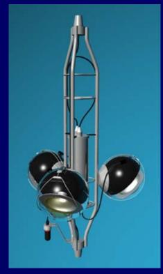
String-based PMT sat downward 45° at 2500 m deep
